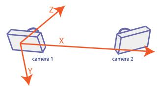
In a stereo system, the origin is located at the optical center of Camera 1.
