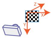
When you reconstruct a 3-D scene from multiple views containing a calibration pattern, the resulting 3-D points are defined in the pattern-based coordinate system. The "Structure From Motion From Two Views" example shows how to reconstruct a 3-D scene from a pair of 2-D images containing a checkerboard pattern.
