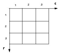
For pixel coordinates, the number of rows, r, downward, while the number of columns, c, increase to the right. Pixel coordinates are integer values and range from 1 to the length of the row or column. The pixel coordinates used in Computer Vision Toolbox software are one-based, consistent with the pixel coordinates used by Image Processing Toolbox<sup>™</sup> and MATLAB. For more information on the pixel coordinate system, see "Pixel Indices" (Image Processing Toolbox).
